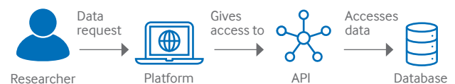
Figure 6: Overview of the process for obtaining data access via the research API.
